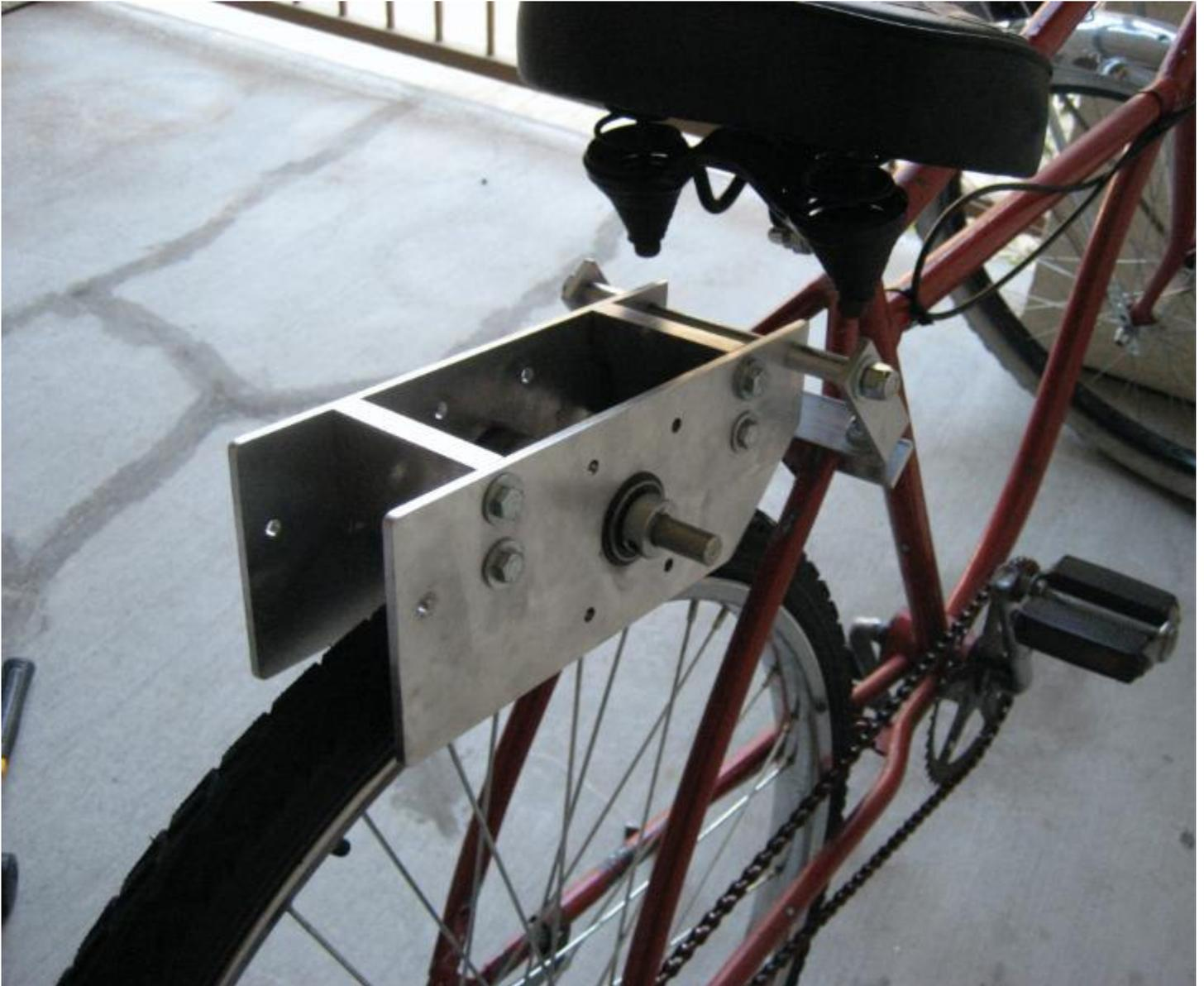
The picture above shows the front support bracket mounted to the bicycle. Notice the low profile of the bracket. The Staton front support bracket makes the engine channel sit up a bit taller than mine. The shorter front support bracket makes it more stable and less susceptible to bending.
