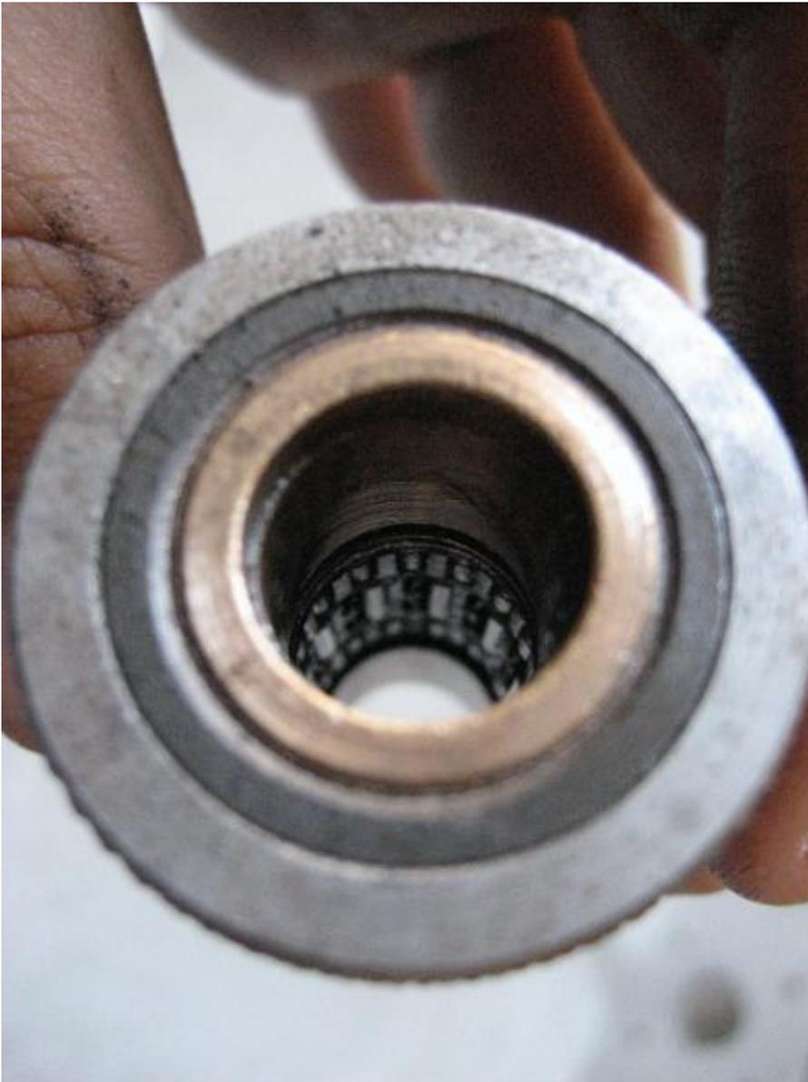
I also made a couple of shaft collars to center the drive roller on the drive shaft.
