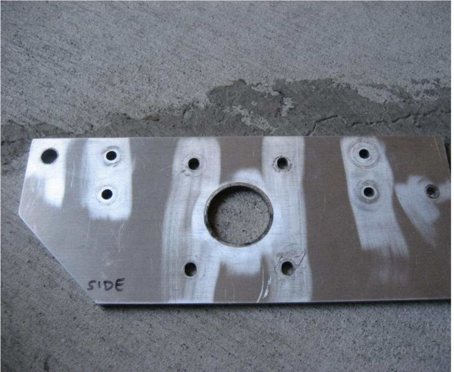
After cutting everything out on the mill, I put the engine channel together using some  $\frac{1}{4}$ " bolts. Notice that I made the engine channel a bit narrower than the Staton engine channel. The Staton channel is 4" wide and mine is 3.5" wide. I made it narrower so that the engine would not come out as far. By moving it in  $\frac{1}{4}$ ", it would decrease the torsional force that is produced by having load on one side.
