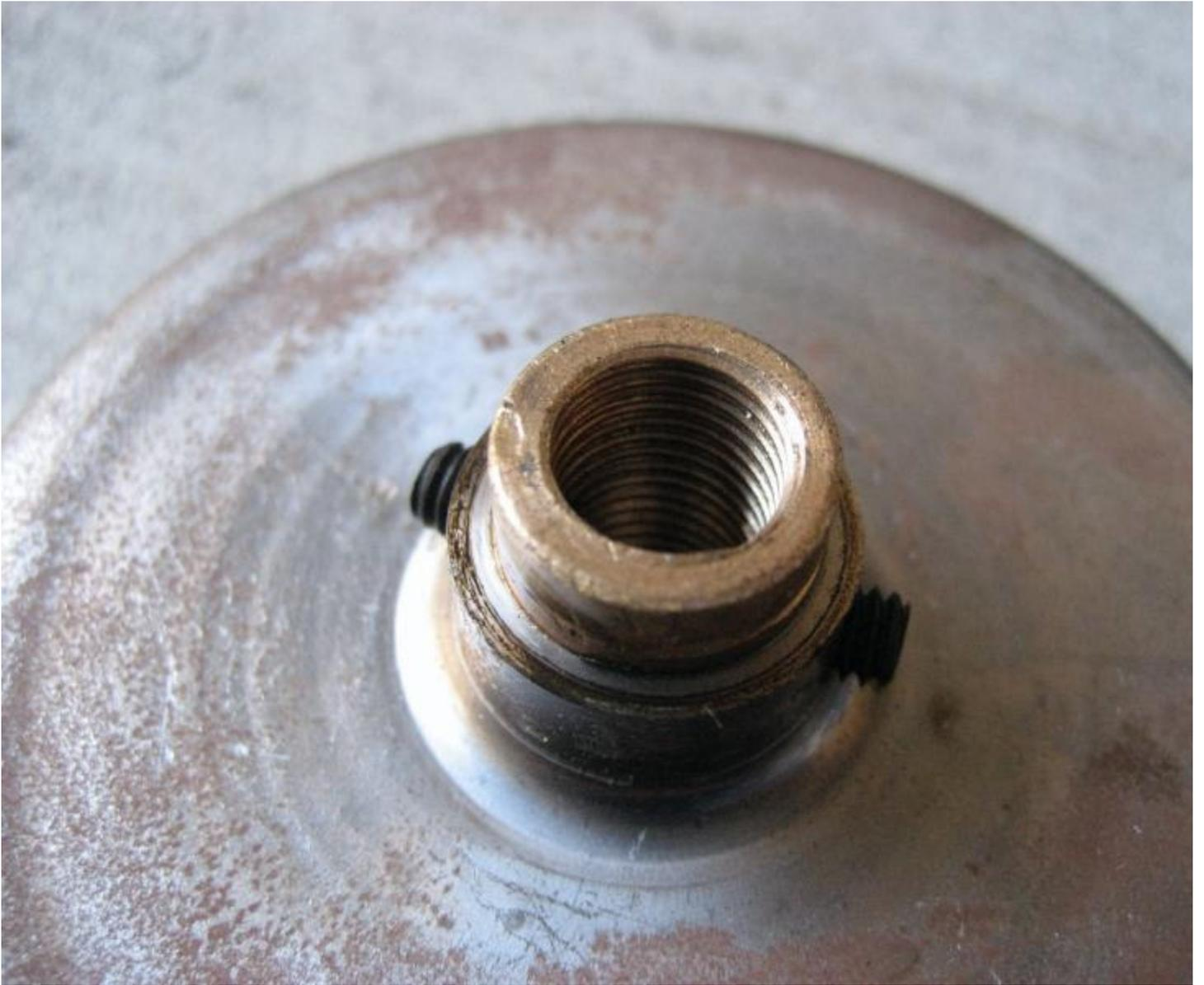
The modified clutch drum will not fit over the original clutch rotor with the roller drive shaft in place because there is an extension of the engine drive shaft where the clutch drum used to screw onto. I had to cut off this extension on the engine drive shaft so that the clutch drum would fit nicely over the clutch rotor.
