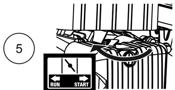
**IMPORTANT:** Allow the engine to run at no load for five minutes with no load after each start-up so that the engine can stabilize.
